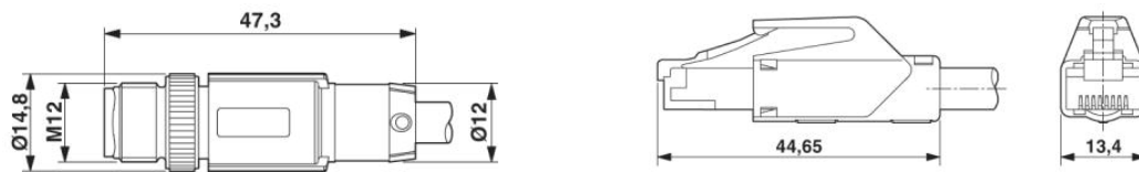
M12 x 1 male connector, straight, shielded
